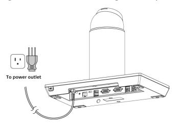
1. To use the premium docking station, firstly connect the AC adapter to the DC-in input and connect the other end to the power outlet. Always plug in the AC adapter first to enable the locking/unlocking function.
